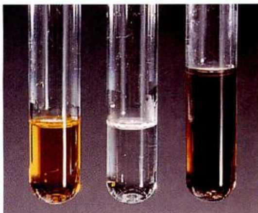
Figure 21.2 The redox reaction between dichromate ion and iodide ion. When \text{Cr}_2\text{O}_7^{2-} (left) and \text{I}^- (center) are mixed in acid solution, they react to form \text{Cr}^{3+} and \text{I}_2 (right).
